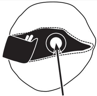
j) Ensure the green cap in the end of the capsule is clear of any obstructions. The pouch is now ready to be stowed in the tube. Close the pouch using the velcro.
