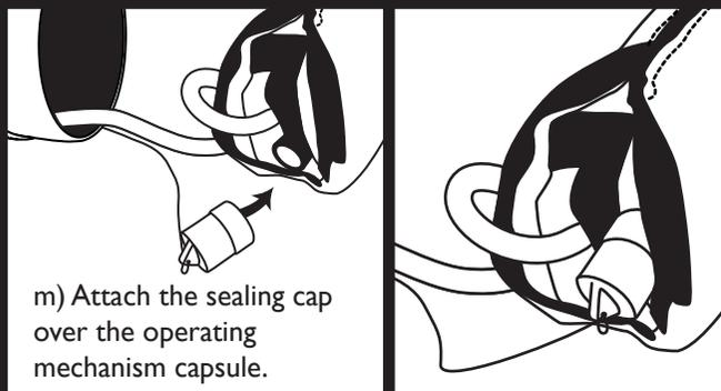
m) Attach the sealing cap over the operating mechanism capsule.
