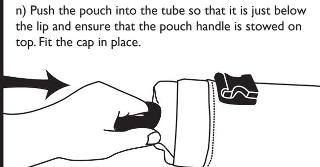
n) Push the pouch into the tube so that it is just below the lip and ensure that the pouch handle is stowed on top. Fit the cap in place.
